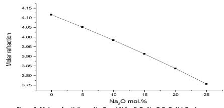
Figure 2: Molar refractivity vs. Na<sub>2</sub>O mol.% for B<sub>2</sub>O<sub>3</sub>-Na<sub>2</sub>O-ZnO- Nd<sub>2</sub>O<sub>3</sub> glasses
