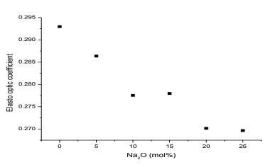
Figure 7: Elasto optic coefficient vs. Na<sub>2</sub>O mol.% for B<sub>2</sub>O<sub>3</sub>-Na<sub>2</sub>O-ZnO- Nd<sub>2</sub>O<sub>3</sub> glasses
