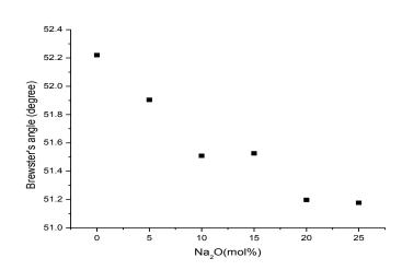
Figure 9: The Brewster's angle vs. Na<sub>2</sub>O mol.% for B<sub>2</sub>O<sub>3</sub>-Na<sub>2</sub>O-ZnO- Nd<sub>2</sub>O<sub>3</sub> glasses
