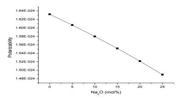
Figure 6: Polarizability vs. Na<sub>2</sub>O mol.% for B<sub>2</sub>O<sub>3</sub>-Na<sub>2</sub>O-ZnO- Nd<sub>2</sub>O<sub>3</sub> glasses
