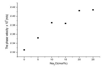
Figure 10: The speed of light of the medium vs. Na<sub>2</sub>O mol.% for B<sub>2</sub>O<sub>3</sub>-Na<sub>2</sub>O-ZnO- Nd<sub>2</sub>O<sub>3</sub> glasses
