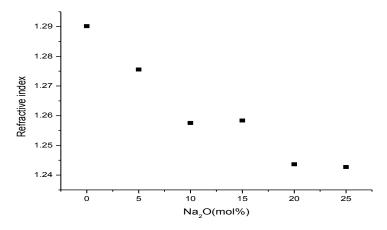
Figure 3: Refractive index vs. Na<sub>2</sub>O mol.% for B<sub>2</sub>O<sub>3</sub>-Na<sub>2</sub>O-ZnO- Nd<sub>2</sub>O<sub>3</sub> glasses
