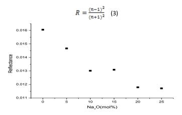
Figure 4: reflectance vs. Na<sub>2</sub>O mol.% for B<sub>2</sub>O<sub>3</sub>-Na<sub>2</sub>O-ZnO- Nd<sub>2</sub>O<sub>3</sub> glasses
