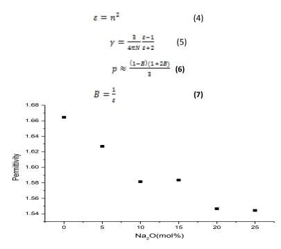
Figure 5: Permittivity vs. Na<sub>2</sub>O mol.% for B<sub>2</sub>O<sub>3</sub>-Na<sub>2</sub>O-ZnO- Nd<sub>2</sub>O<sub>3</sub> glasses
